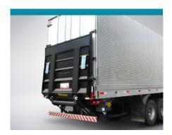
For various applications (palletised cargos, hand carts, rolltainers and pushcarts), with a cargo capacity of between 400 and 2500kg,
